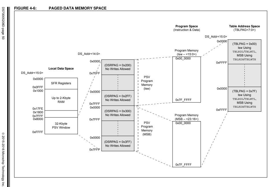
When a PSV page overflow or underflow occurs, EA<15> is cleared as a result of the register indirect EA calculation. An overflow or underflow of the EA in the PSV pages can occur at the page boundaries when:
