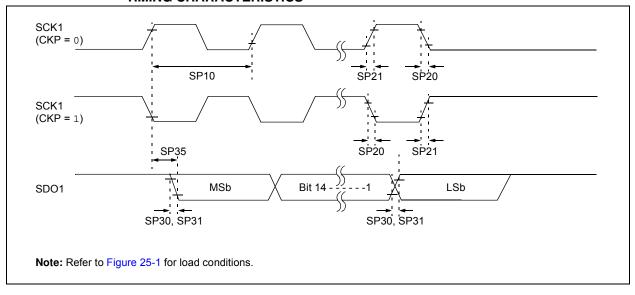
FIGURE 25-12: SPI1 MASTER MODE (HALF-DUPLEX, TRANSMIT ONLY, CKE = 1) TIMING CHARACTERISTICS
